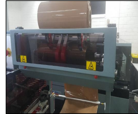
Photo 5: WRAPPER SLCT-FA16004: Perforation wheels behind closed interlocked guard
