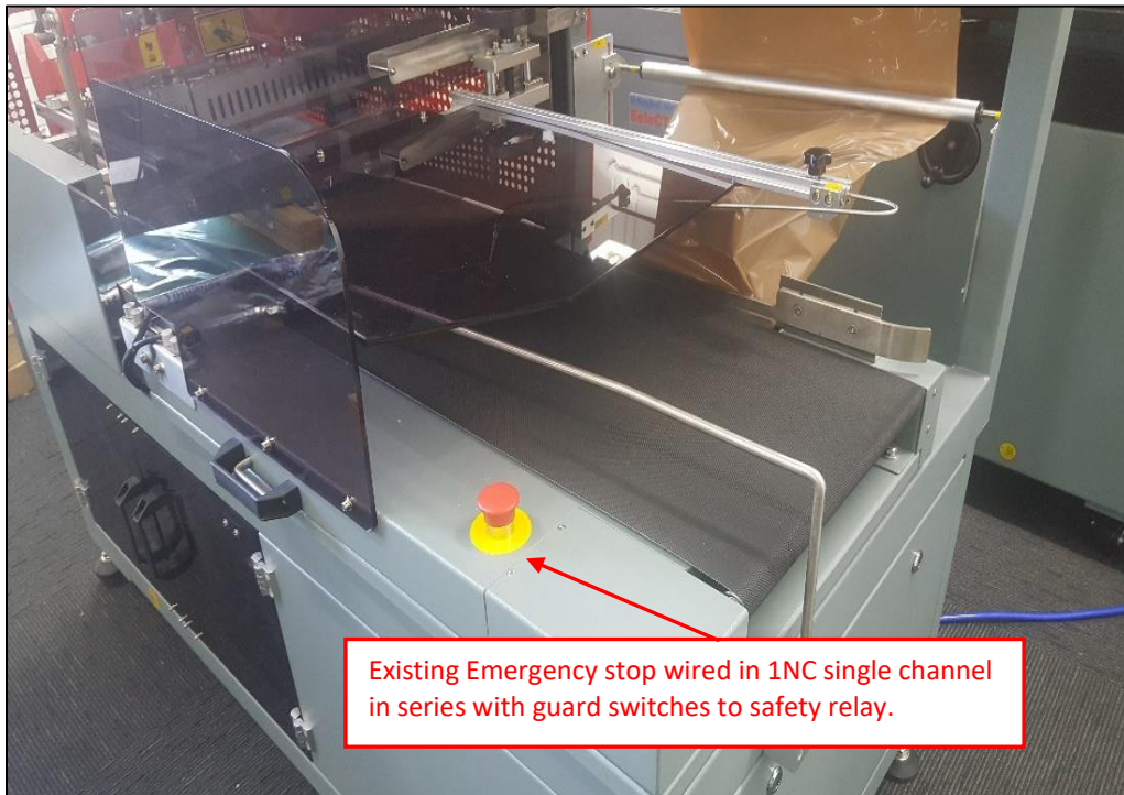
Photo 10: Wrapper SLCT-FA16004: Emergency stop near infeed conveyor
